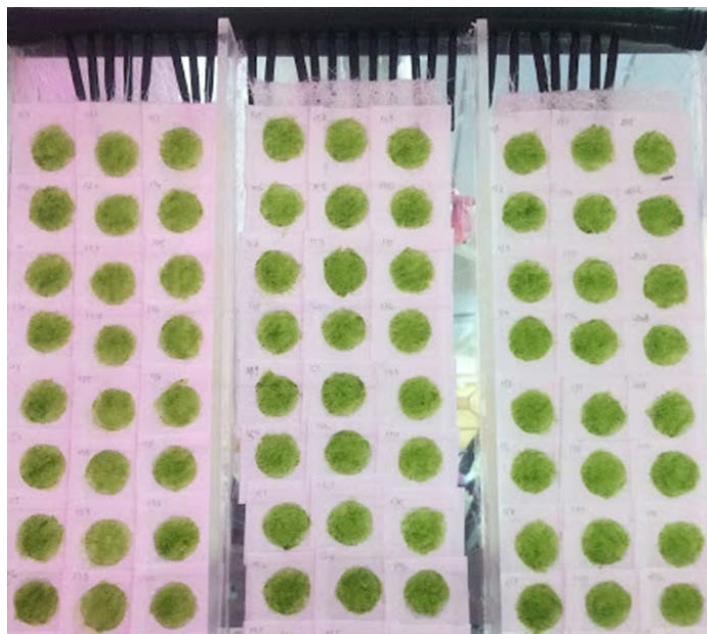
Figure 4. Microalgae C. vulgaris after immobilisation in biofilm PBR
